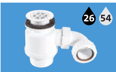
50mm Water Seal Resealing Trap with 1½" Multifit Outlet Overall height 118mm
