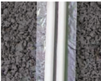
Fig. 38 Metallic tape can be used to aid electronic pipe detection
