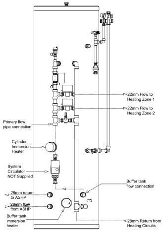
Figure 3-1: Pre-plumbed cylinder (buffer option)
