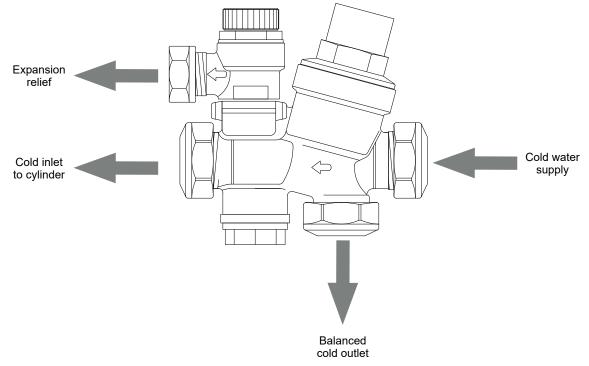
Figure 4-1: Cold water inlet manifold
