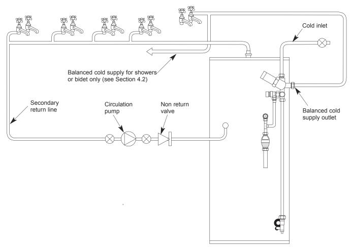
Figure 4-2: Secondary return circuit
