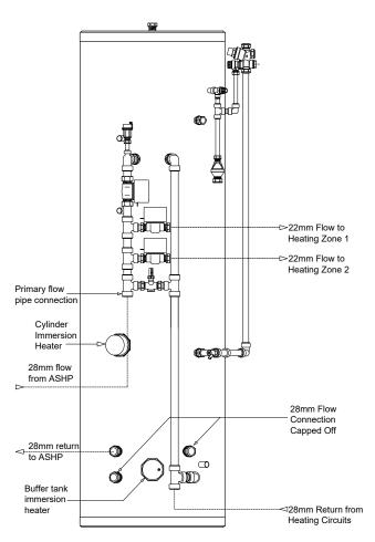
Figure 3-2: Pre-plumbed cylinder (volumiser option)
