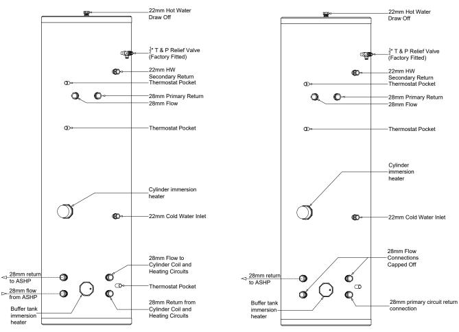
Figure 3-3: Standard cylinder (buffer option)
