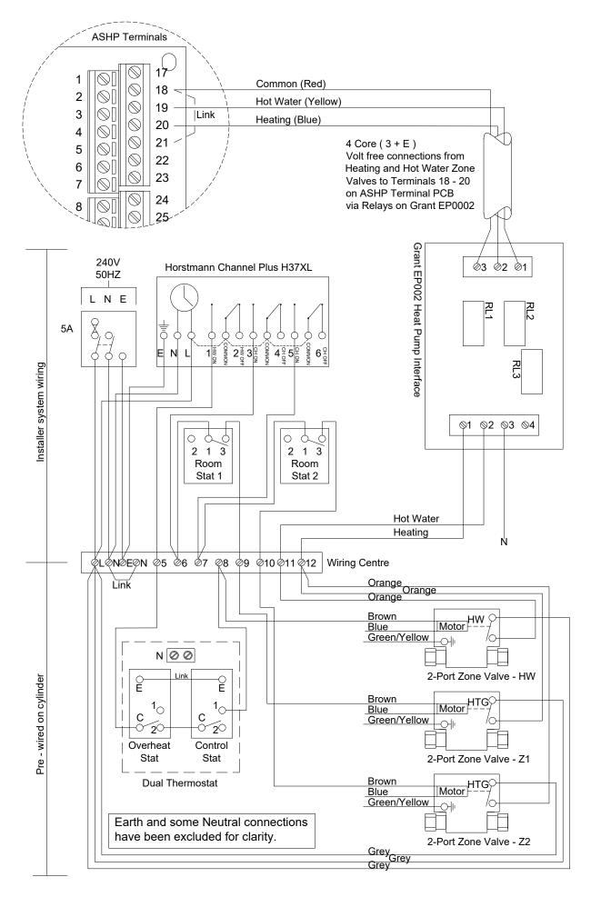
Figure 5-3: Pre-plumbed cylinder (volumiser option)
