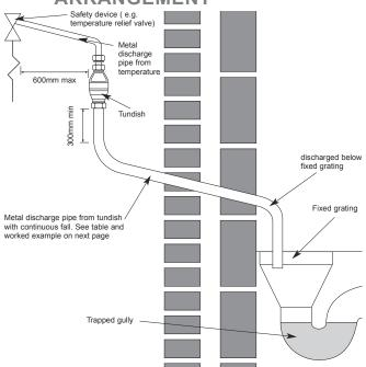
Figure 4-2: Typical discharge pipe arrangement
