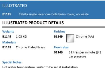
Hot water temperature limiter to be set at installation. Regulated flow rate 5 litres per minute at 1 bar.
