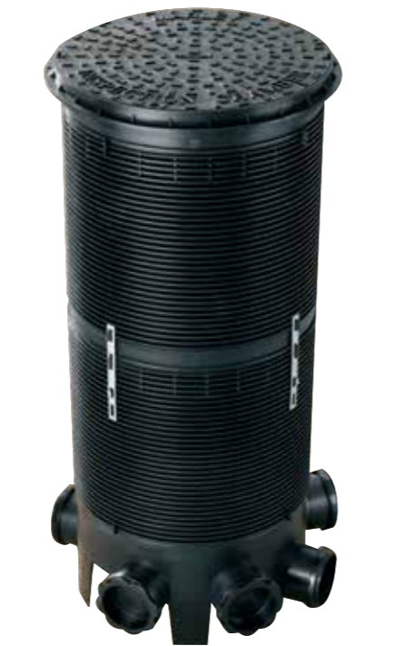
Deep inspection chamber 450x110mm chamber base (UCC3D), riser (UCR3), access ring (UCLRR), lid (UCL35PP) & clip (UCC10D)
