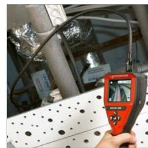
Camera head with high-performance LEDs
