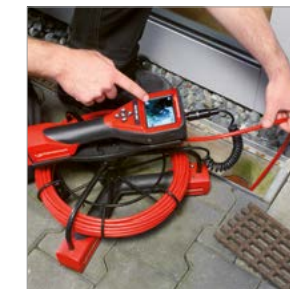
Inspection of rain drainpipes
