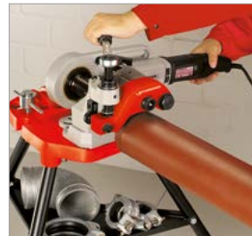
Use with roll grooving tool ROGROOVER
