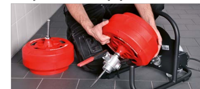
Interchangeable drum for different working ranges
