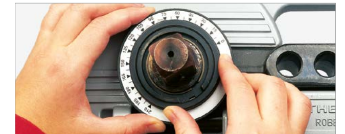
Pre-adjustment of the bending angle without tools
