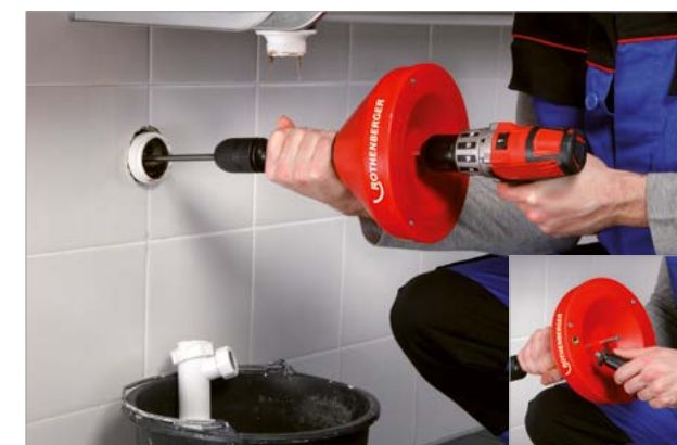
Electrical operation with cordless drill
