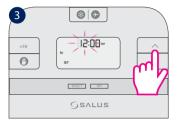
Press UP or DOWN to select the hour Press UP or DOWN to select the minutes and then press SELECT to confirm your and then press SELECT to confirm your option. option.
