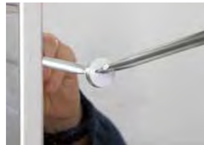
LOCK Lock the cabinet securely in place using the locking button
