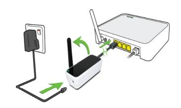
Connect the gateway to your router. Gateway is online when the green LED is on.
