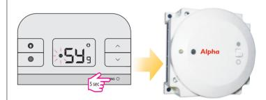
**4.** The countdown on the thermostat's screen will continue. Once the pairing process is successful, there is no need for you to wait for the the countdown to stop. To return to normal display, press and hold the Test/Sync button on your thermostat for 5 seconds.
