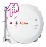
2. Press and hold the Test/Sync button on your thermostat for 5 seconds then release. The thermostat should display words "SYNC 9". A 9 minute countdown will appear on thermostat's screen.
