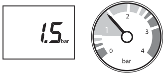
Fig.52 Restore water pressure
