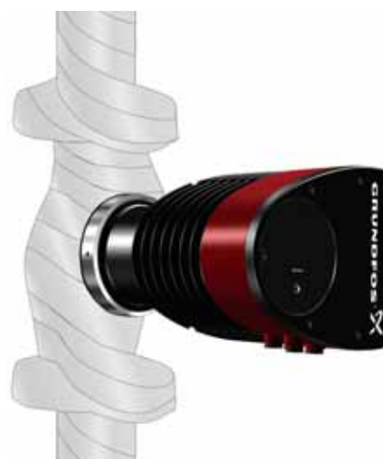
Fig. 9 Insulation of the pump housing and pipe
