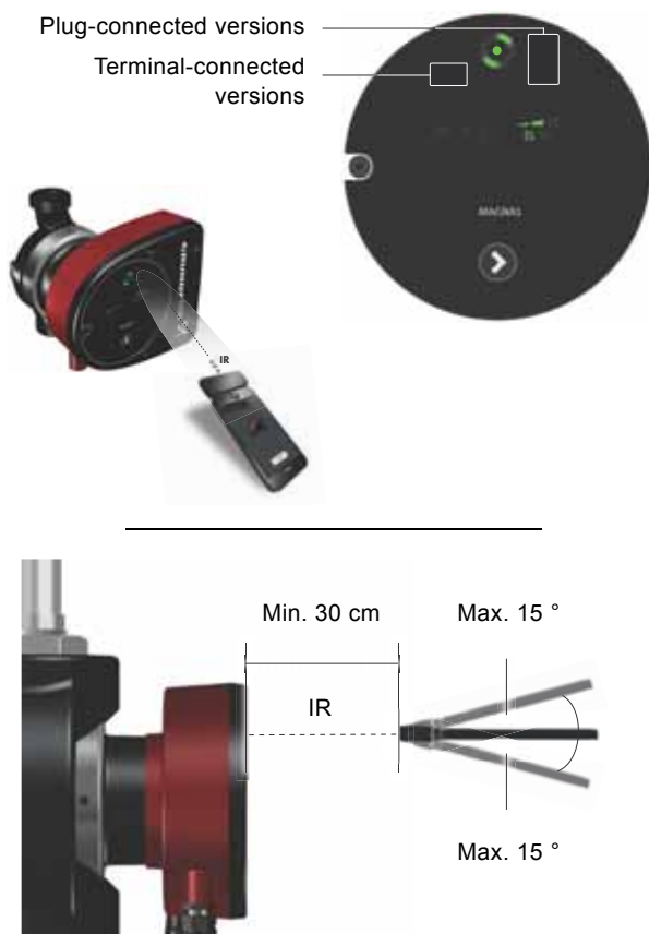
Fig. 31 Establishing a connection between Grundfos GO and MAGNA1 via infrared communication
