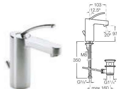
5A3046C00 Monobloc basin mixer with aerator, pop-up waste and 3/8" flexible supply hoses
