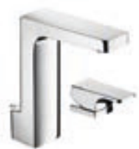
5A3801C00 Monobloc basin mixer with 8 l/min flow limiter, separate deck-mounted handle, aerator, pop-up waste and 3/8" flexible supply hoses
