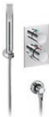
5A2762C00 1/2" built-in thermostatic bath-shower mixer with diverter-flow regulator to supply 1/2" wall-mounted bath filler, 1.7m flexible shower hose, handset, fixed bracket and 1/2" water connection
