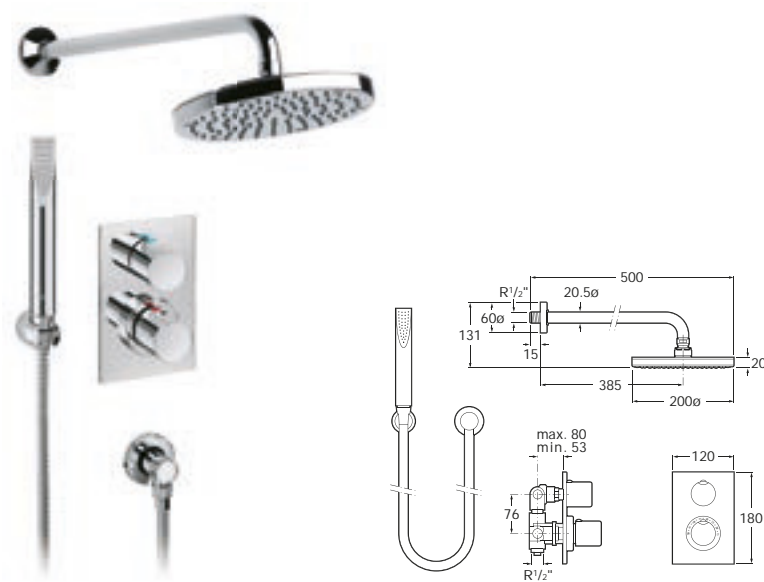
5A2962C00 1/2" built-in thermostatic shower mixer with diverter-flow regulator to supply shower arm, movable high-flow shower head, 1.7m flexible shower hose, handset, fixed bracket and 1/2" water connection
