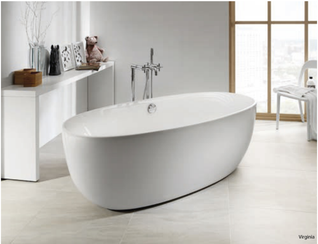
248313000 ⊗ 1700 x 800 One-piece acrylic bath with integrated panel and pop-up waste. Supplied with adjustable legs. For freestanding installation. Capacity: 175 litres up to overflow
