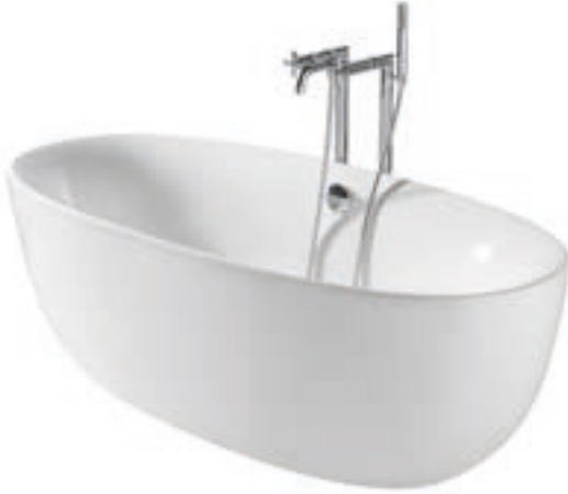
248313000 ⊗ 1700 x 800 One-piece acrylic bath with integrated panel and pop-up waste. Supplied with adjustable legs. For freestanding installation. Capacity: 175 litres up to overflow
