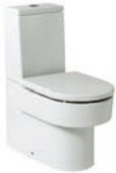
342567000 Box-rim WC pan dual outlet with V0007600R floor fixing kit (moulded back-to-wall) 341567000 Cistern complete with 822806001 6/3 litre dual-flush cistern fittings (left hand water supply only) 801562004 Lacquered soft-close seat and cover
