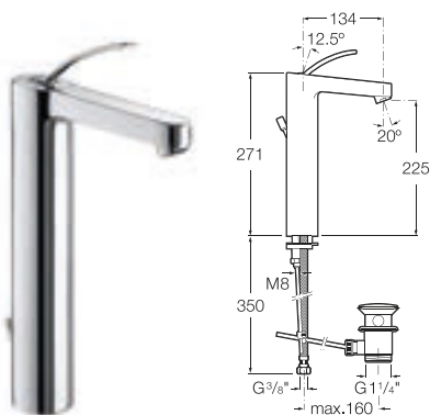
5A3446C00 Extended monobloc basin mixer with aerator, pop-up waste and 3/8" flexible supply hoses
