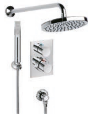
5A2962C00 1/2" built-in thermostatic shower mixer with diverter-flow regulator to supply shower arm, movable high-flow shower head with pivot, 1.7m flexible shower hose, handset, fixed bracket and 1/2" water connection
