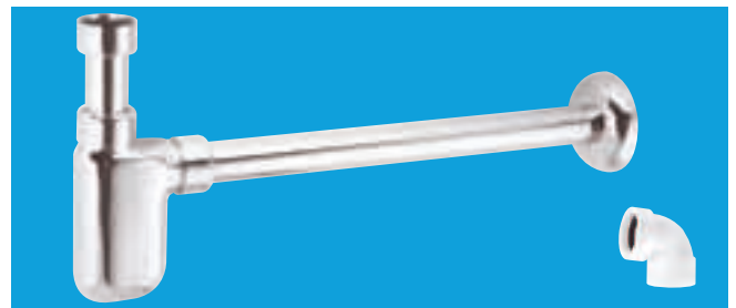
1 1/4" x 75mm Water Seal Brass Adjustable Inlet Bottle Trap with 16" length of 32mm OD CP brass waste pipe and wall flange
