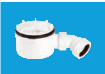
50mm Water Seal Trap Body with 1½" Multifit outlet. Adjustable height 105-168mm. Flow rate 34 l/min*
