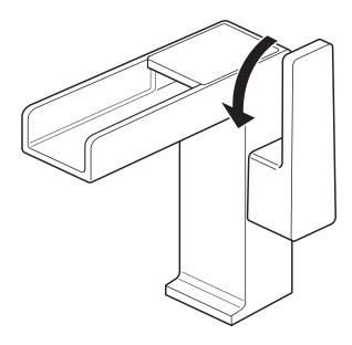
Moving the mixer lever forwards will actuate the flow of water and progressively increase the water temperature.
