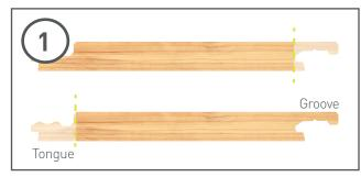
Hydrolock panels are supplied as standard with a tongued long edge and a grooved long edge. When fitting panels into an extrusion, the protruding tongued or grooved edge should be cut off.
