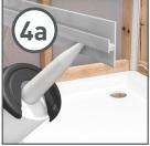
Apply silicone sealant to the channel of the second profile and attach it to the long edge of first panel.
