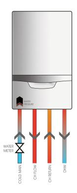
As the water in the cold main begins to warm, the expanding water volume begins to put increasing pressure on system components, increasing the chance of failure and leaks.
