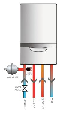
With the inta MINIM shock arrestor kit installed between the water meter and boiler, system components are protected as the expanded water volume is harmlessly absorbed by the shock arrestor.
