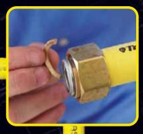
**4. Fit AutoFlare® Fitting**Place the AutoFlare® fitting into the back nut & engage threads. Note that the AutoFlare® fitting is designed to form a metal-onmetal leak-tight seat on the piping as you tighten the fitting. No paste should be used. Using appropriate wrenches, tighten the fitting until the resistance to wrenching increases greatly. The flare has now been created on the piping end.
