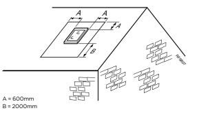
The flue terminal shall not penetrate the shaded area of the roof.
