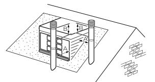
If chimney penetrates dotted area such that A is less than 300mm, B shall not be less than 300mm.
