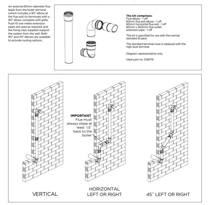
If additional elbows to those supplied in the High Level Flue Outlet kit are used, deduct the following resistances (metres) from the maximum boiler flue length.
