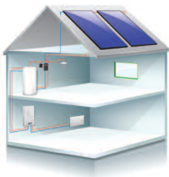
Zenith solar system Mynute i sealed system boiler Aquaflow unvented twin coil cylinder
