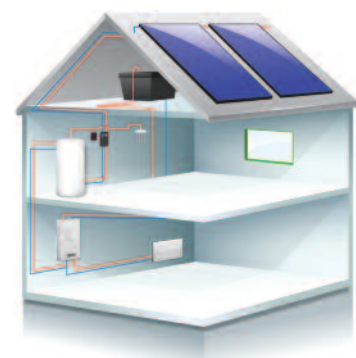
Zenith Solar system Mynute VHE regular open vent boiler Aquaflow unvented twin coil cylinder
