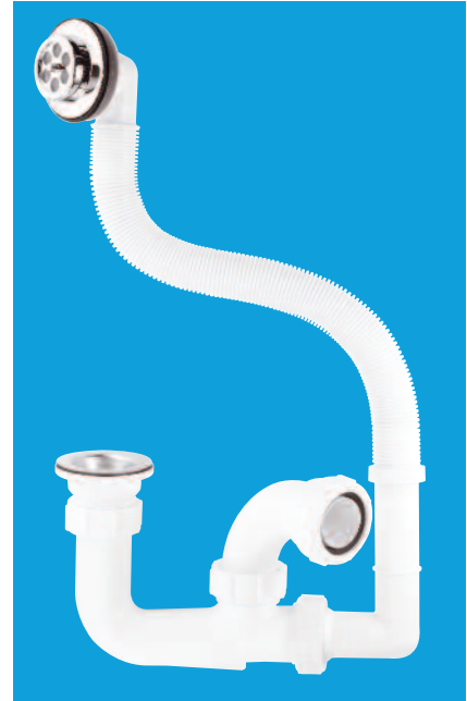
1½" x 75mm Water Seal with flexible overflow tube and CP overflow grating and 70mm flange centre pin waste outlet fitting
