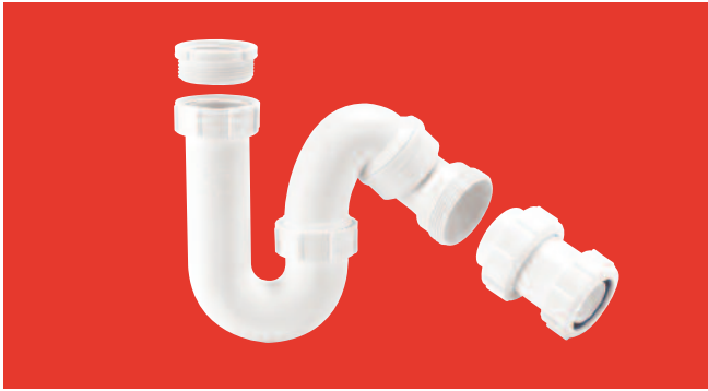
Tubular HandiTrap 75mm water seal with 1 1/4" and 1 1/2" inlets and outlets. Note: Trap outlet can be swivelled from 'P' to 'S' position
