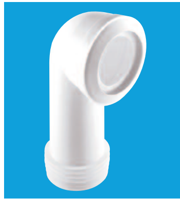
90° Bend (Long) 97-107mm Inlet 4"/110mm Outlet
