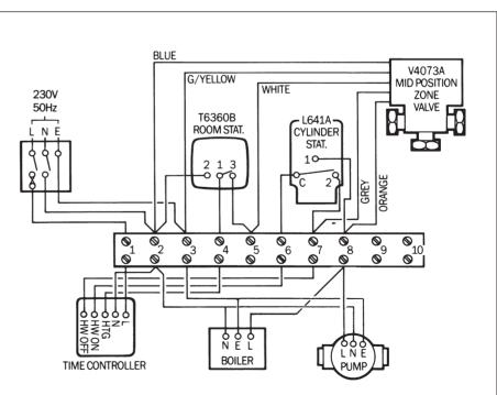
Note: It is recommended that the 10 way Junction Box or Sundial Wiring Centre should be used to ensure first time, fault free wiring.
