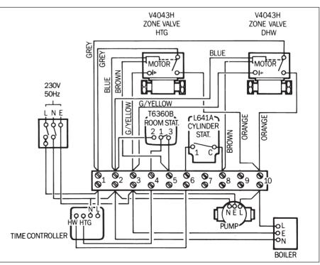
Note: It is recommended that either the 10 way Junction Box or Sundial Wiring Centre should be used to ensure first time, fault free wiring.
