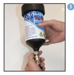
Fit the drain valve assembly to the bottom of the Mag Defender making sure the outlet is at the front of the assembly and being careful not to overtighten as this may cause damage.
