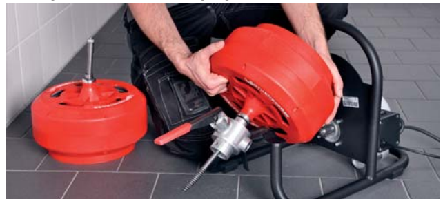
Interchangeable drum for different working ranges
