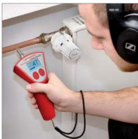
Acoustic Leak detection of heating installations
