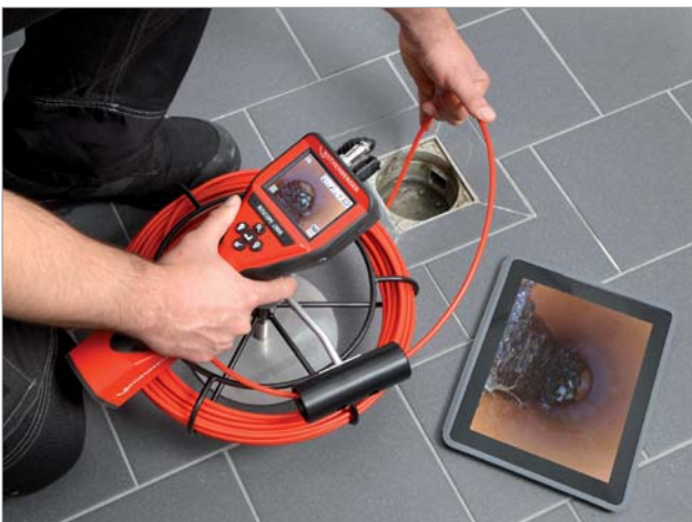
Inspection of basin drains
