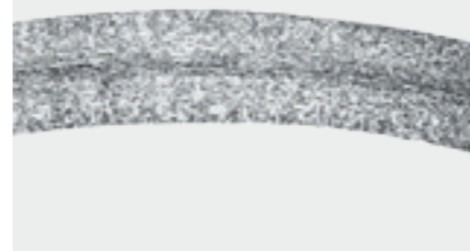
Exact spheroidisation of the seal ring for long-term tightness and high mechanical strength.
