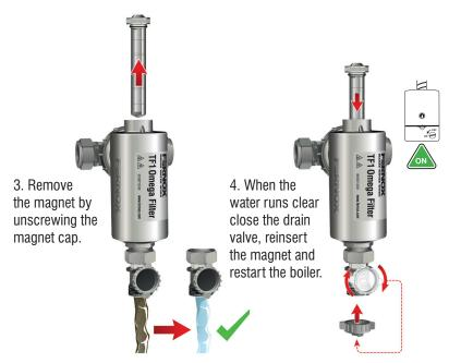
Ensure that the magnet sheath remains clean and dry.
