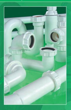
Traps to BS EN 274-1:2002 are manufactured in white high temperature polypropylene with compression type outlets that fit plastic and copper waste pipes 32mm/1¼" and 40mm/1½".
