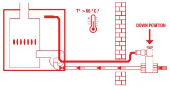
The effect of excessive heat on the sensor causes the valve to close tightly, thus preventing the main storage tank from fuelling the fire.
