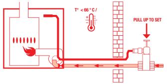
When fitted to the oil supply line, the Remote Acting Fire Valve from EPS can help to prevent total destruction by fire.
