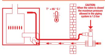
The valve will not re-open unless the manual reset is activated, this must be attempted only once the fire risk has been eliminated.
