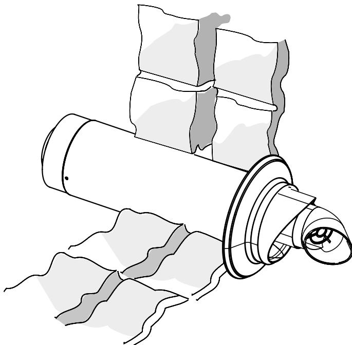
**NOTE: FLUE DEFLECTOR TO BE ANGLED TO THE LEFT OR RIGHT ONLY - NOT UP OR DOWN, TO PREVENT RAIN INGRESS**
