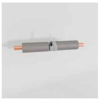
Apply insulation on both sides as far as the clamp and wrap round with CLIMAFLEX® PE selfadhesive tape up to the insulation level.
