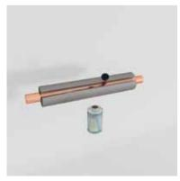
... fit round the pipe, spread the two surfaces of the slit with a thin coat of NMC-FIX®, and press the insulation together after allowing the regulation time for the adhesive to dry (finger test). For problem areas, such as screwed fittings, we recommend fastening with a few clips.
