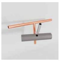
Punch out the T-shaped branches using the punch in the slit area ...
