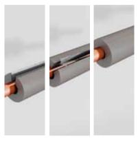
Fit CLIMAFLEX® XT round the pipe, tear off both protective sheets simultaneously and press the insulation together.
