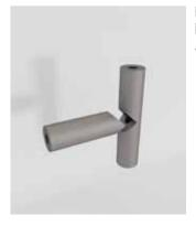
In the case of T-shaped branches, cut a T at a 45-degree angle ...
