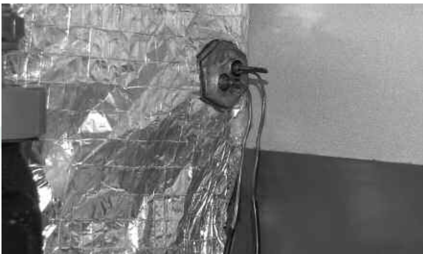
Figure 10-3: Thermostat phial position
