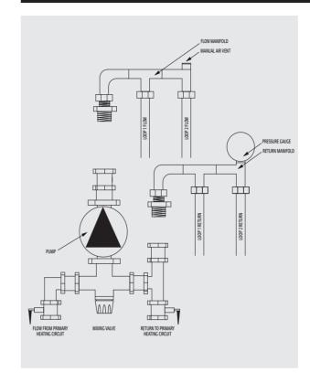
If only one heating loop is used, cap off the second loose connection with the supplied fitting.
