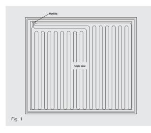
The two-port manifold is installed at a convenient location in, or near the area to be heated. The heating pipework is connected to the flow manifold (which contains the air vent) and then laid out in the required configuration. Pipes are held in place with a clip rail system, which is fixed with self-adhesive strips to a separation membrane (supplied and laid by others) placed over the insulation (supplied and laid by others).
