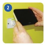
After first ensuring that the bracket is secure, clip the iT500 into place by aligning the recess on the back of the unit to the bracket and clipping into place.
