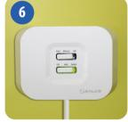
When the iT500RX Receiver and the iT500 Thermostat are paired then the light will be green.
