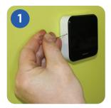
To pair the iT300 to the receiver, insert a paperclip or similar object into the hole on the left hand side of the iT300 for 2 seconds.
