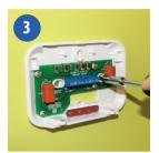
Fit the back of the receiver unit to the wall using the fittings supplied.
