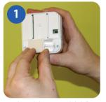
Remove the battery cover on the back of the iT300 unit.
