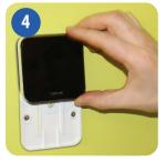
Align the grooves on the back of the iT300 unit and slide onto the bracket.
