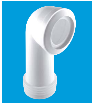
90° Bend (Long) 90-112mm Inlet 4"/110mm Outlet
