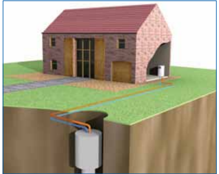
Example of bore hole collector system
