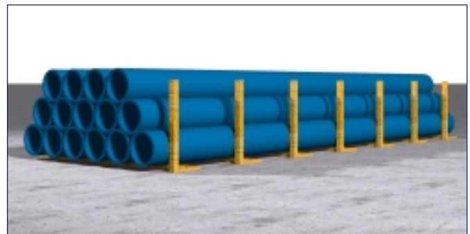
Figure 32. Loose Pipe Storage
