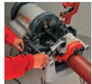
Cost-effective production of grooves
