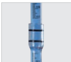
Transparent tube element with double o-ring seal
