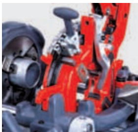
Automatic die head with integrated oil supply
