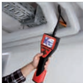
Inspection of hollow spaces
