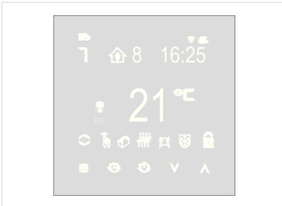
Smart Thermostat to control room temperature from in house or via smart device. The MU-050 is completely smooth fronted with soft touch icons for control and energy efficiency.
