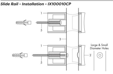
The screws and wall plugs supplied are only suitable for use in solid walls. If the wall is plaster board or soft building block use special wall plugs obtainable from most DIY stores.
