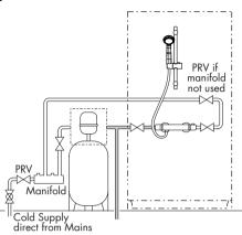
Flow regulators are required for installations where a PRV is not fitted to ensure simultaneous demand is accounted for.
