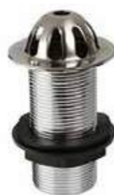
Stainless Steel Urinal Waste STAINLESS STEEL REMOVABLE DOME COVER Brass Body 3/4" Tail Length 2 1/2" Flange Size
