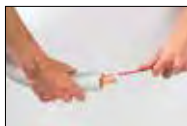
STEP 1 Insert the flexible bender of the right diameter into the copper tube.
