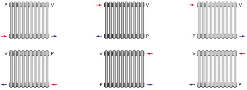
NB: Bottom opposite end connection is recommended for 2000mm high radiators.
