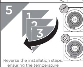
stop is aligned correctly.
