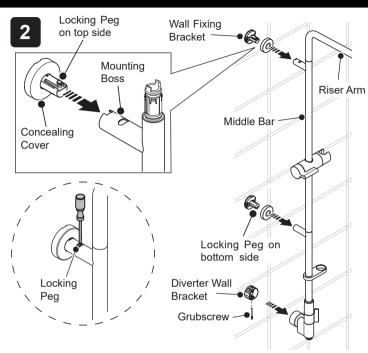
Loosen and remove the grubscrew to pull off the diverter from wall bracket. Discard the grubscrew.
