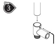
Place the **Riser Rail** into the **Bottom Bracket** (water outlet) and align the holes. Insert the pin and tighten with the supplied allen key.
