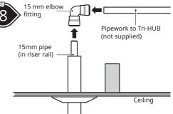
In the loft, trim any excess length of the 15mm pipe.
