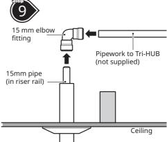
In the loft, trim any excess length of the 15mm pipe.
