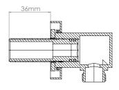
Screw the **Bulkhead Adaptor** to the pipework. Add a bead of silicone sealant around the adaptor to ensure watertight.
