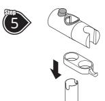
Slide the **Hose Retainer** and then the **Shower Head Holder** onto the **Riser Rail** — press and hold the button on top of the holder to release the locking mechanism, then slide onto the rail.
