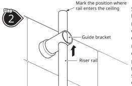
Slide the **Riser Rail** up through the **Guide Bracket** until it touches the ceiling.
