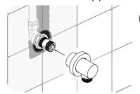
Fit the **Bulkhead** onto the **Adaptor** and retighten the grub screws.
