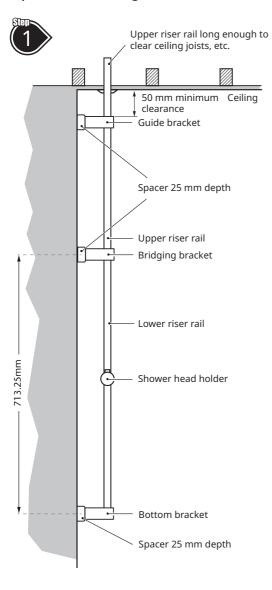
The 940mm & 700mm Riser Rails are supplied to cater for differing layouts and ceiling heights. It may be necessary to shorten one of the rail sections using a suitable hacksaw or pipe cutter.
