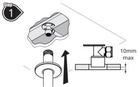
Install a wall plate elbow or suitable alternative with a minimum of 3 fixing screws, ensuring that the flush fitting pipework has suitable support.
