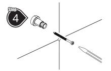
Slide the Hose Retainer, Shower Head Holder and then the Top Bracket on to the Riser Rail, offer the Riser Rail up to the wall, align vertically and mark the screw hole.
