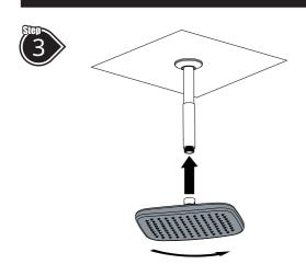
Assemble the **Fixed Head** on to the **Ceiling Arm.**
