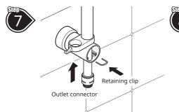
Feed the 15mm pipe and connector back up the Riser Rail and secure the Outlet Connector with the Retaining Clip.
