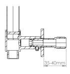
Screw the **Adaptor** to pipework.
