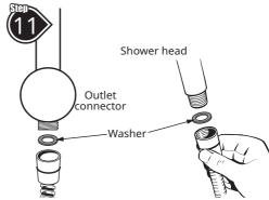
Screw the **Shower Hose** to the **Outlet Connector** and the other end to the **Shower Head**.
