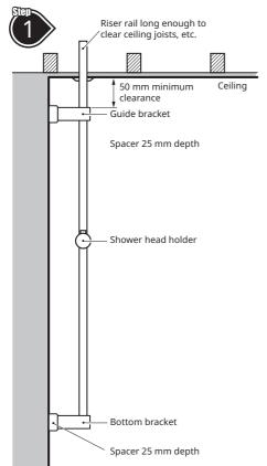
Allow a minimum distance of 50mm between the ceiling and the **Guide Bracket**. Make sure there is sufficient length of **Riser Rail** above the ceiling level to overcome any obstructions to running the water pipe down the **Riser Rail**, such as the height of the ceiling joist.
