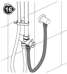
Take the **Short Hose** and fit a hose seal into the conical nut and connect to the **Bulkhead**, fit a hose seal into the conical nut at the other end of the hose and connect to the inlet of the **Diverter Valve**.
