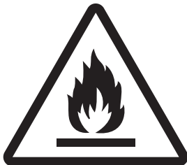
Caution: Risk of fire/flammable materials
