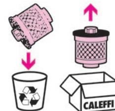
The damaged cartridge and/or strainer screen should be disposed of in a suitable manner.
