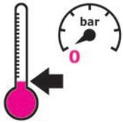
Assembly and disassembly should always be carried out while the system is cold and not under pressure.
