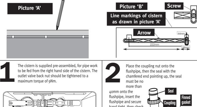
flushpipe and secure hand tight, then check for leaks. Fit the finned gasket as shown, insert into WC and check for leaks.
