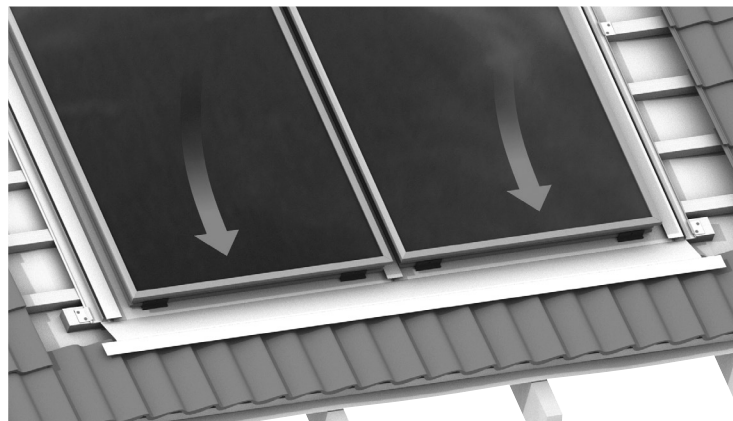
Figure 6-24: Installation of the Collectors on to Bracket
