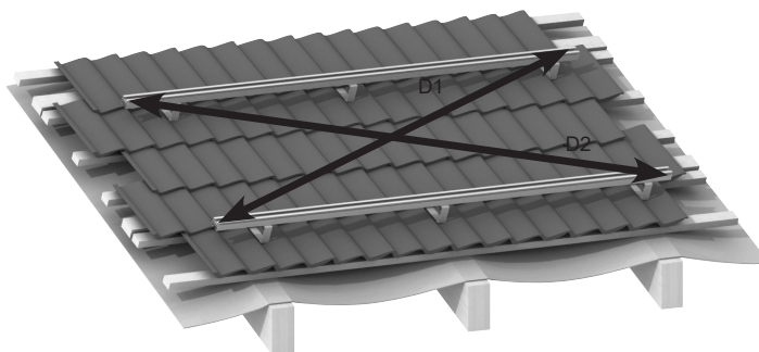
Figure 4-15: Aligning the Mounting Rail
