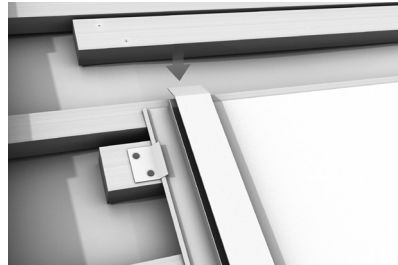
Figure 6-20: Installation of Cover Sheets
