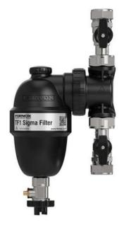
A high-performance, magnetic in-line system filter, the TF1 Sigma Filter is ideal for restricted spaces as it is capable of multiple orientations. This simple to install, composite plastic filter fits onto vertical and horizontal pipework, and works by allowing hydrocyclonic action to deliver contaminants to the unit's powerful magnet assembly for safe removal.
